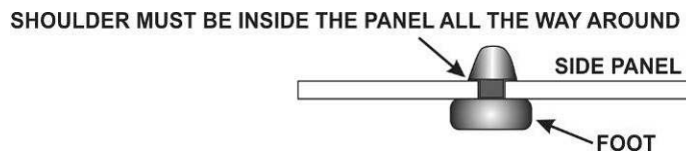
Figure 13. Side Panel Foot Installation.
