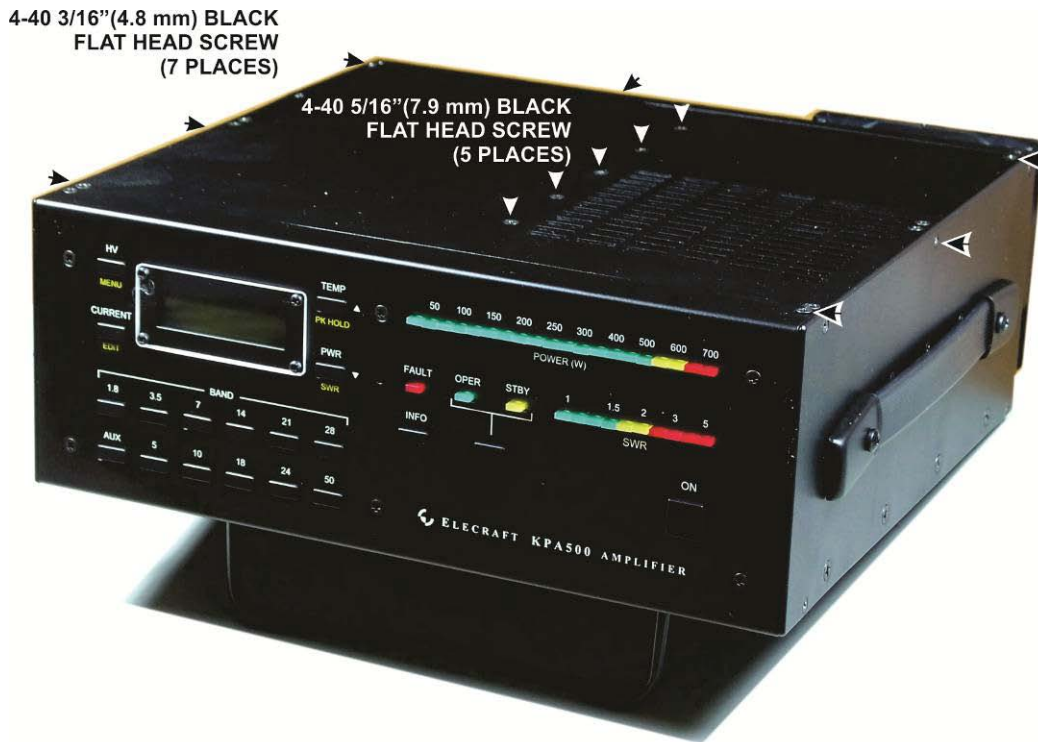
Figure 64. Top Cover Installation.
