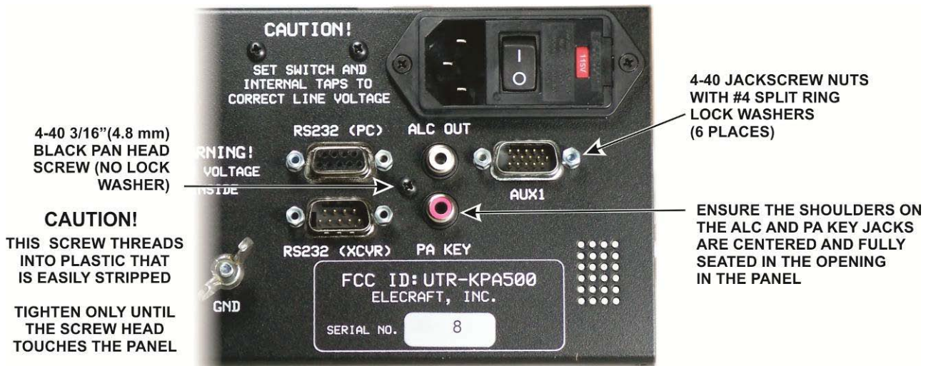
Figure 25. Installing the I/O Module in the Rear Panel.
