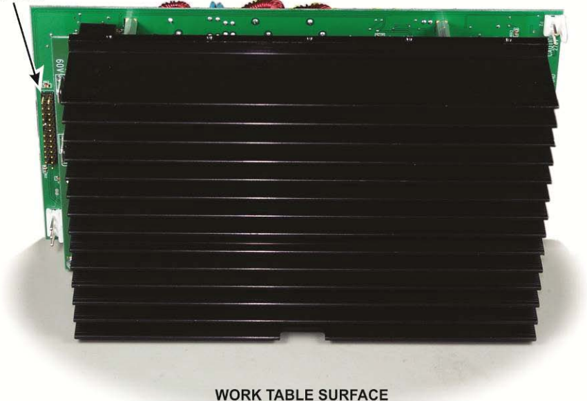
Figure 26. Placing the PA/LPF on the Work Table.
