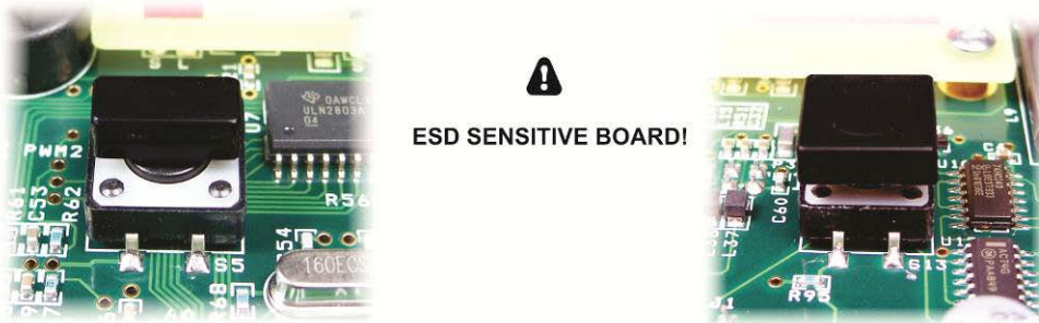
Figure 57. Installing Key Caps on Front Panel Board.
