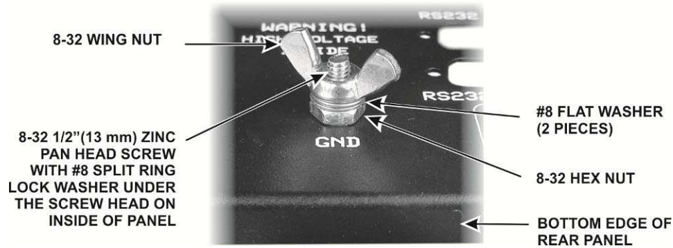
Figure 21. Installing the Rear Panel Ground Lug.
